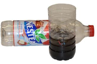
**Fuel** can be mud (low power), 1-2:1 mud/waste water mixture (medium power) or mud/food waste - such as potatoes and meat (highest power). It must be a viscous mass like fresh honey. If needed add tap water or if there is too much water, pour it out. Do not add too much waste water or there will be extensive methane evolution, which reduces efficiency of MFC.
