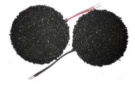
**Electrodes** consist of nanoporous carbon attached onto a special alloy current collector. At least one year of operation has been tested without corrosion and power level is quite stable. Electrodes can be made at home or obtained from superaccu.com. Electrodes are reusable.
