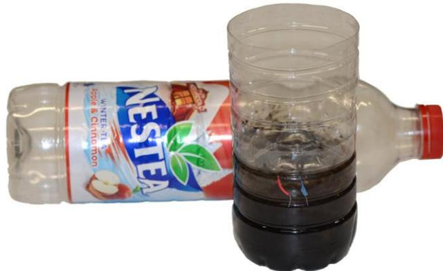
**Fuel** can be mud (low power), 1-2:1 mud/waste water mixture (medium power) or mud/food waste - such as potatoes and meat (highest power). It must be a viscous mass like fresh honey. If needed add tap water or if there is too much water, pour it out. Do not add too much waste water or there will be extensive methane evolution, which reduces efficiency of MFC.
